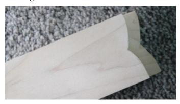
I cannot carve the relief of the blade into the scabbard itself until I know exactly where the blade will rest, so the guard's shape must come first. Once it is filed accurately into one side, I can trace the shape onto the other board and duplicate the filework, resulting in two matching halves.
